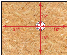
Offset drain location in 34 in. x 42 in. shower area
